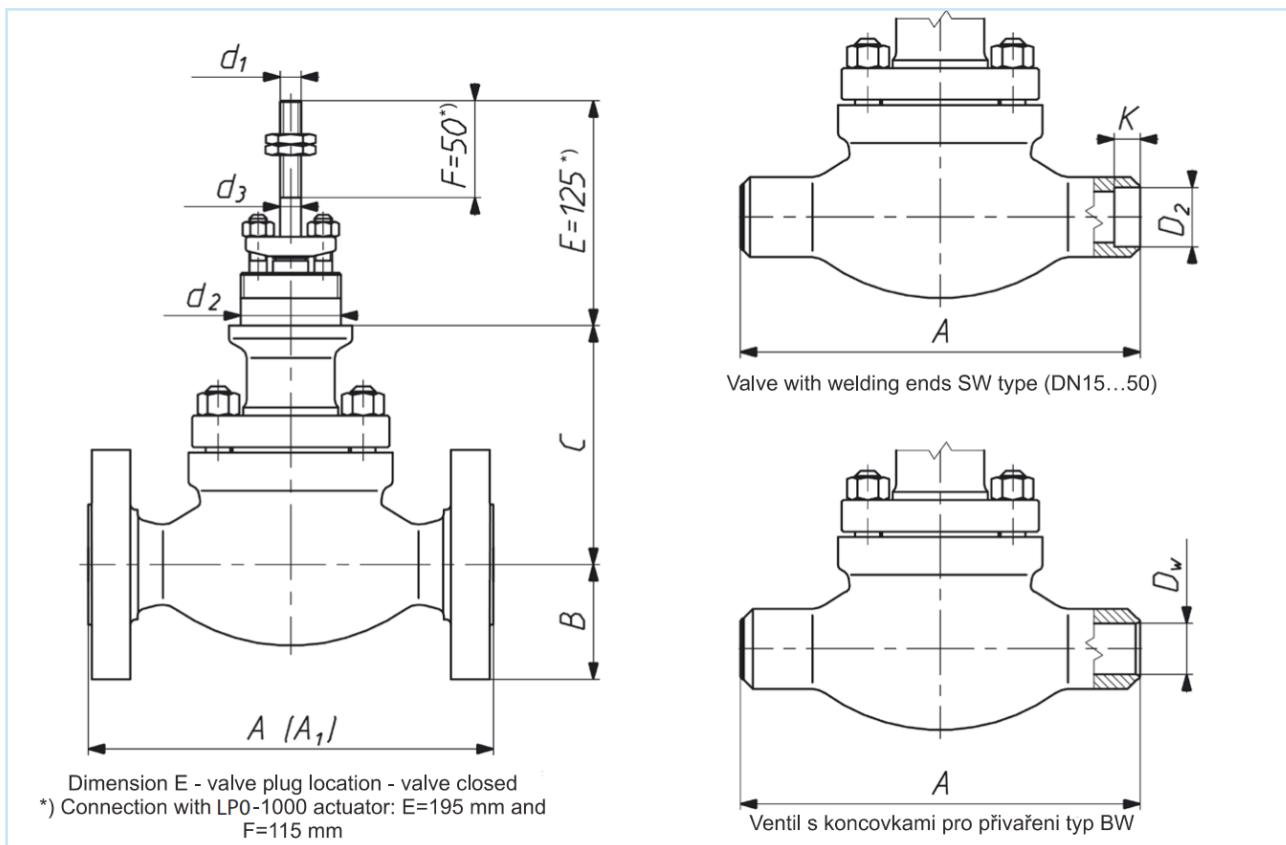
**TABLE 9A - CONNECTION DIMENSIONS OF CONTROL VALVES**
