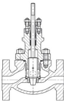
1B - contoured valve plug and choke cage
