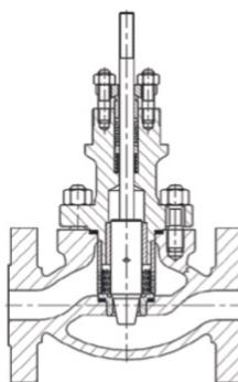
1C - perforated valve plug and compression cage
