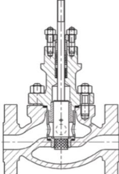
1D - perforated valve plug and choke cage
